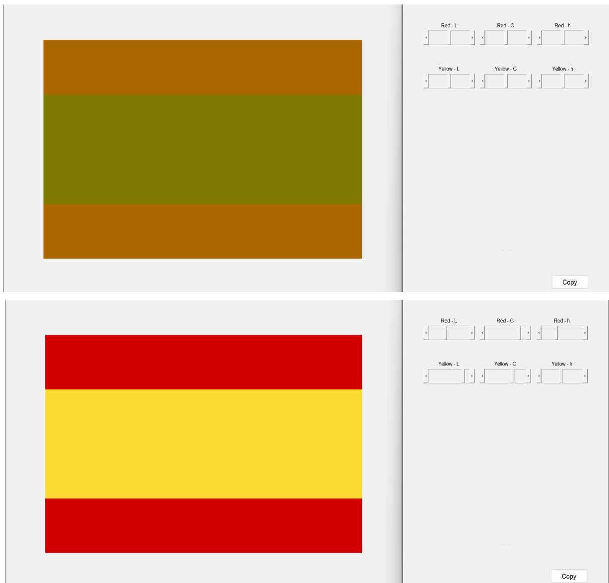
Fig.1. Interface of the software employed in the visual experiment. Upper plot: Observers saw a flag with the legal dimensions of the flag of Spain but with colors that were very different from the official ones [10]. They then had to use the 6 sliders shown on the right side of the screen to perform the requested task. Lower plot: An example of the final flag proposed by an observer after modifying the initial positions of the sliders.
